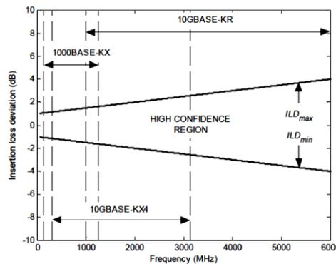
Figure 69B-6—Insertion loss deviation limits
