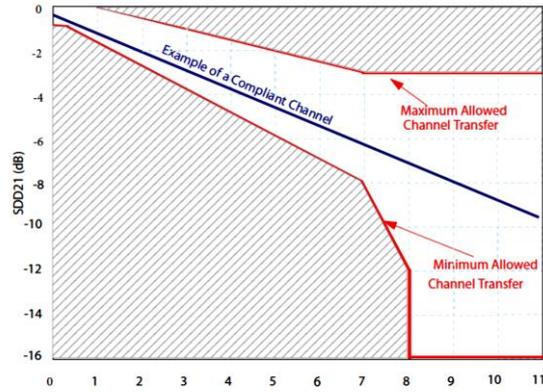
Figure 33 Example of SFI Host Recommended Channel
