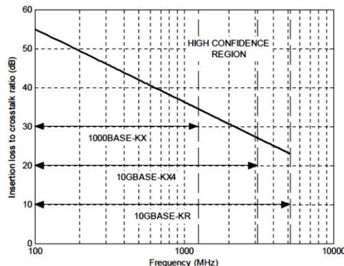
Figure 69B-8—Insertion loss to crosstalk ratio limit
