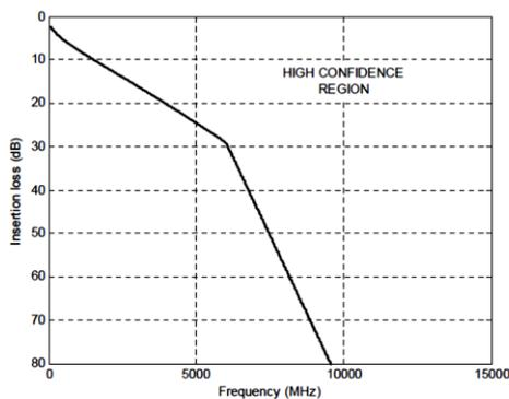
Figure 69B-5—Insertion loss limit for 10GBASE-KR
